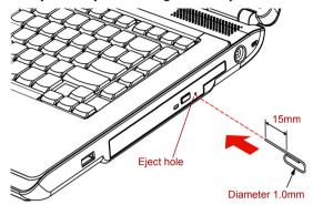
Figure 4-3 Manual release with the eject hole
